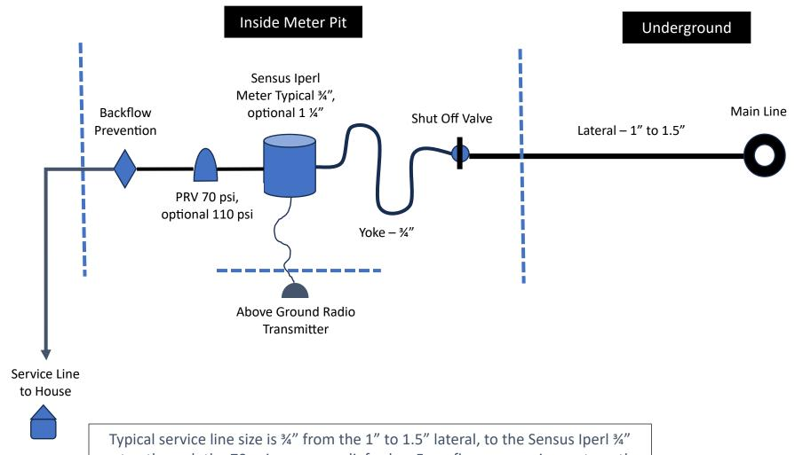
Typical service line size is  $\frac{3}{4}$ " from the 1" to 1.5" lateral, to the Sensus Iperl  $\frac{3}{4}$ " meter, through the 70 psi pressure relief valve. For a fire suppression system, the meter size may be increased to 1  $\frac{1}{4}$ " along with the service line to the house.
